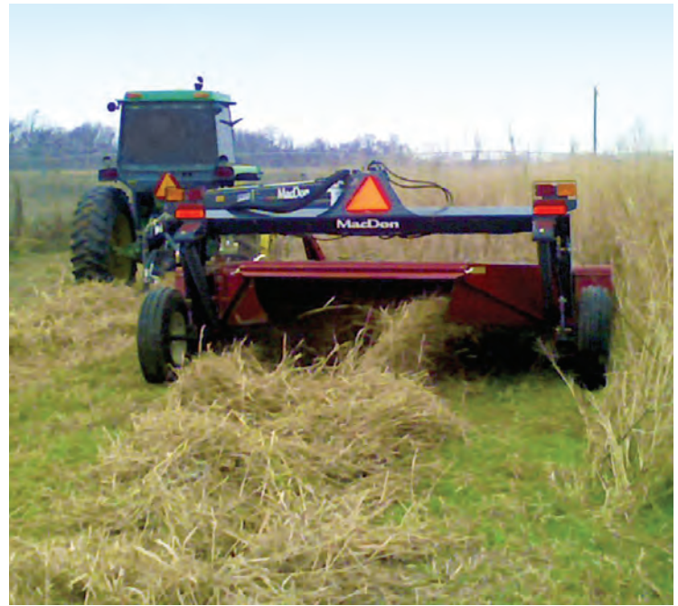
A tractor pulls a MacDon mower-conditioner through a field as it cuts switchgrass.
