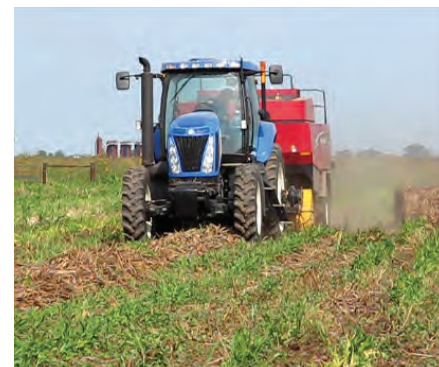
A biomass baler is used to collect harvested crops for storage and transportation.
